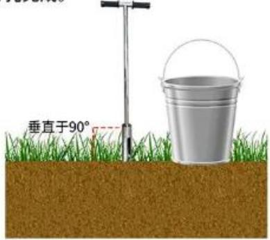
Diagram illustrating the soil drilling process. A hand-operated soil drill is shown being used to create a hole in the ground. A bucket is placed next to the drill. A dashed line indicates the drill is perpendicular to the ground surface, labeled "垂直于90°".
